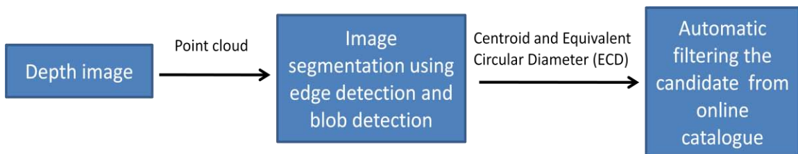
Figure 3.6: Automatic process to filter the 3D space candidates.
