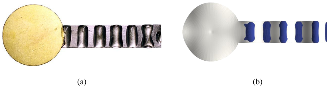
Figure 1. The droplet of vacuum oil on the vibrating plate in the experiment described in [4] (a) and calculated (b), representation longitudinal bending of the vibrating plate, at a scale of 20:1.
