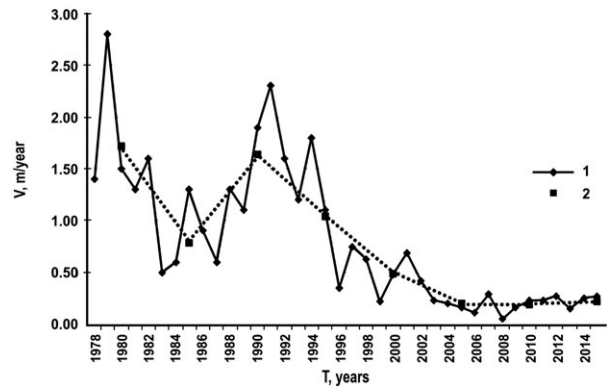
Figure 14. Mean annual gully head retreat rates for the period 1978–2015, based on results of the field monitoring of 168 gully heads in Udmurt Republic (Legend: 1 – mean annual rates; 2 – mean rate over five-year periods; after Rysin et al. , 2017c).
