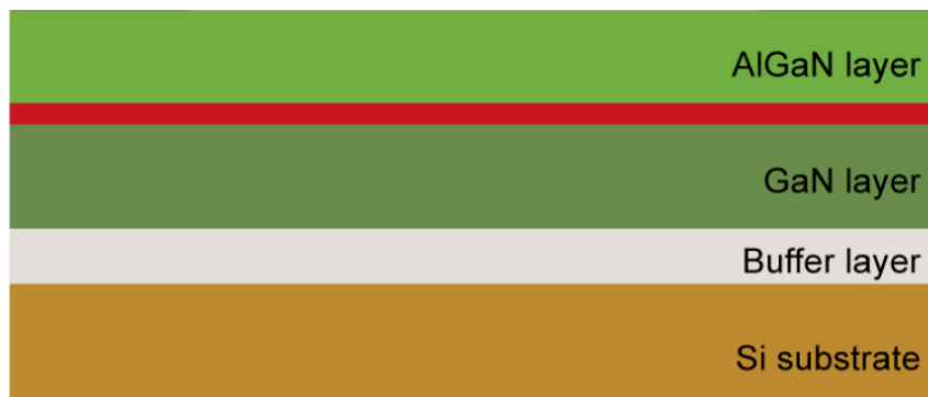
FIG. 3-6 Sketch of GaN on Si with buffer layer
