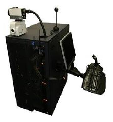
Figure 2.4: Custom thermal imaging system, ATHEMOS. The custom thermal imaging system developed by our group integrates a computer, a thermal camera, and several peripheral hardware components.
