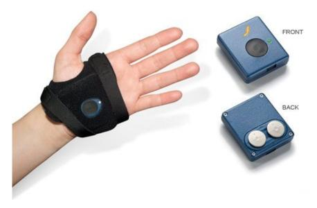
Figure 2.7: The Q Sensor worn on the palm, with the palm strap.
