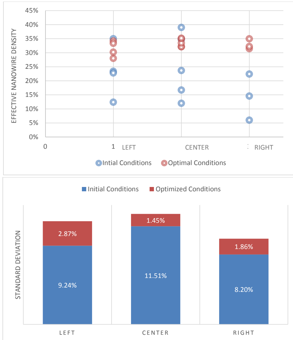
Figure 49: Results from optimized conditions versus initial where (top) optimal conditions show improved reliability and repeatability when targeting NW densities around 30-35% as well as (bottom) reduced growth deviations
