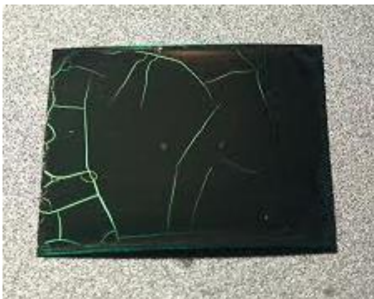
Figure 62: Surface cracking due to thick YBCO films caused by lowering the methanol content in the final precursor solution
