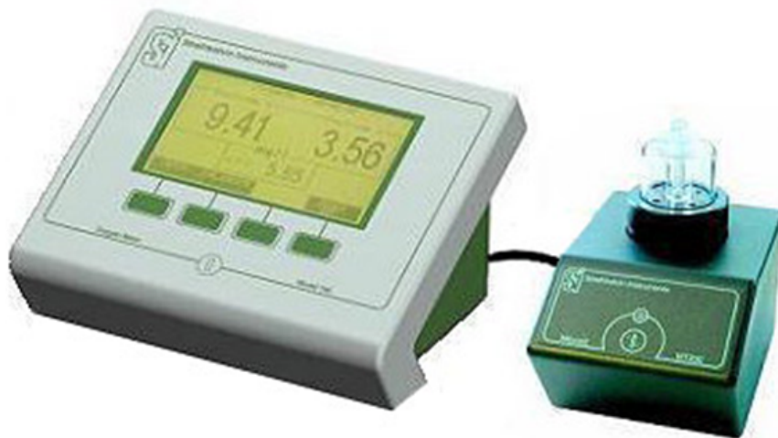
FIGURE 5.10: Mitocell miniature respirometer model MT 200.
