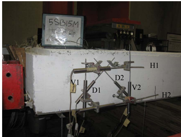
Figure 3.11 Typical LVDT Rosette Installed on the Web of TPSBs
