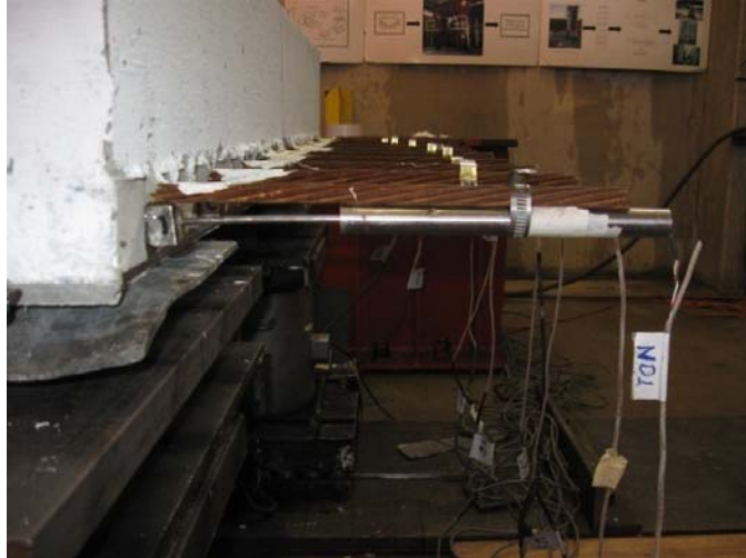
Figure 3.12 LVDTs to Measure End Slip
