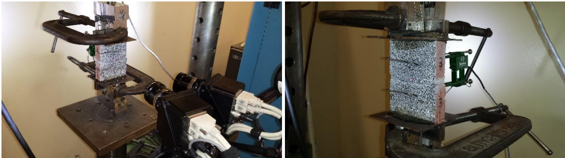
Figure 2-7 Test setup and the two-brick masonry prism specimen for the direct tensile test.
