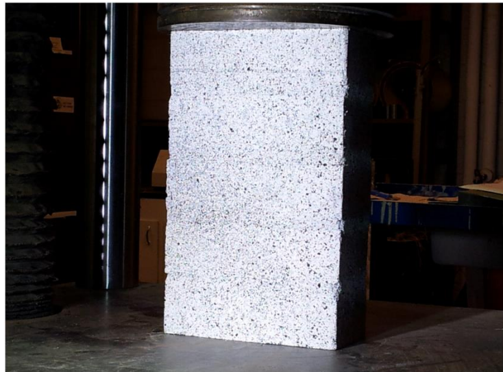
Figure 2-1 Stochastic patterns sprayed on a masonry prism surface.
