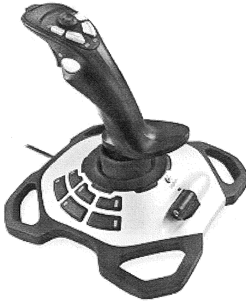
Figure 23: Joystick used to manually control the gimbal and SONY camera. Courtesy: http://ecx.images-amazon.com/images/I/414X2Z0A7TL._SL500_AA280_.jpg
