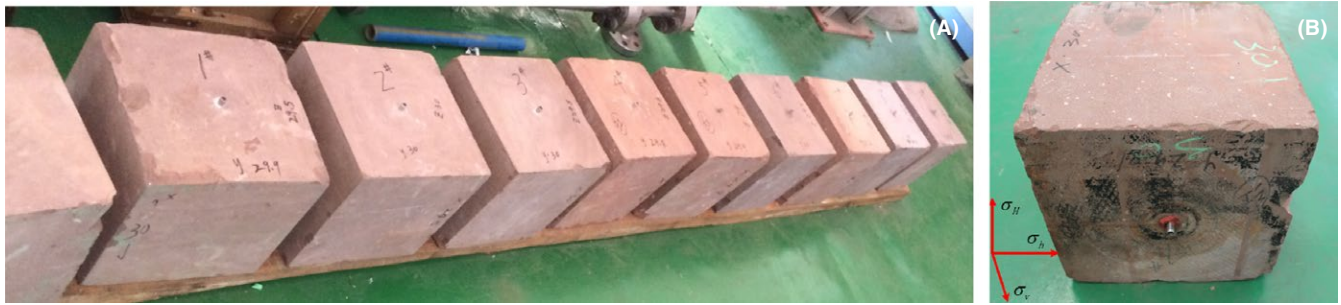
FIGURE 5 The rock samples of Jixi Fault outcrop used in large-scale true triaxial fracturing lab test
