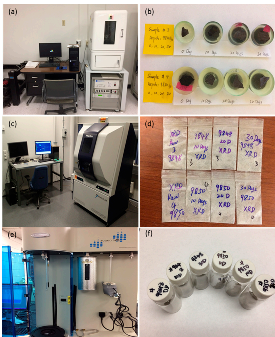
Figure 2. Analysis instruments and samples preparation for the miscellaneous test. (a) Nano-indenter; (b) Sample specimens for the nano-indentation test; (c) X-ray diffraction (XRD); (d) Samples for XRD; (e) Quantachrome Autosorb-IQ; (f) Sample powder for low-temperature N 2 adsorption.
