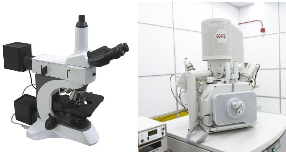
Figure 37 Optical microscopic (left) and SEM (right) to capture the microstructure of the alloy [6].
