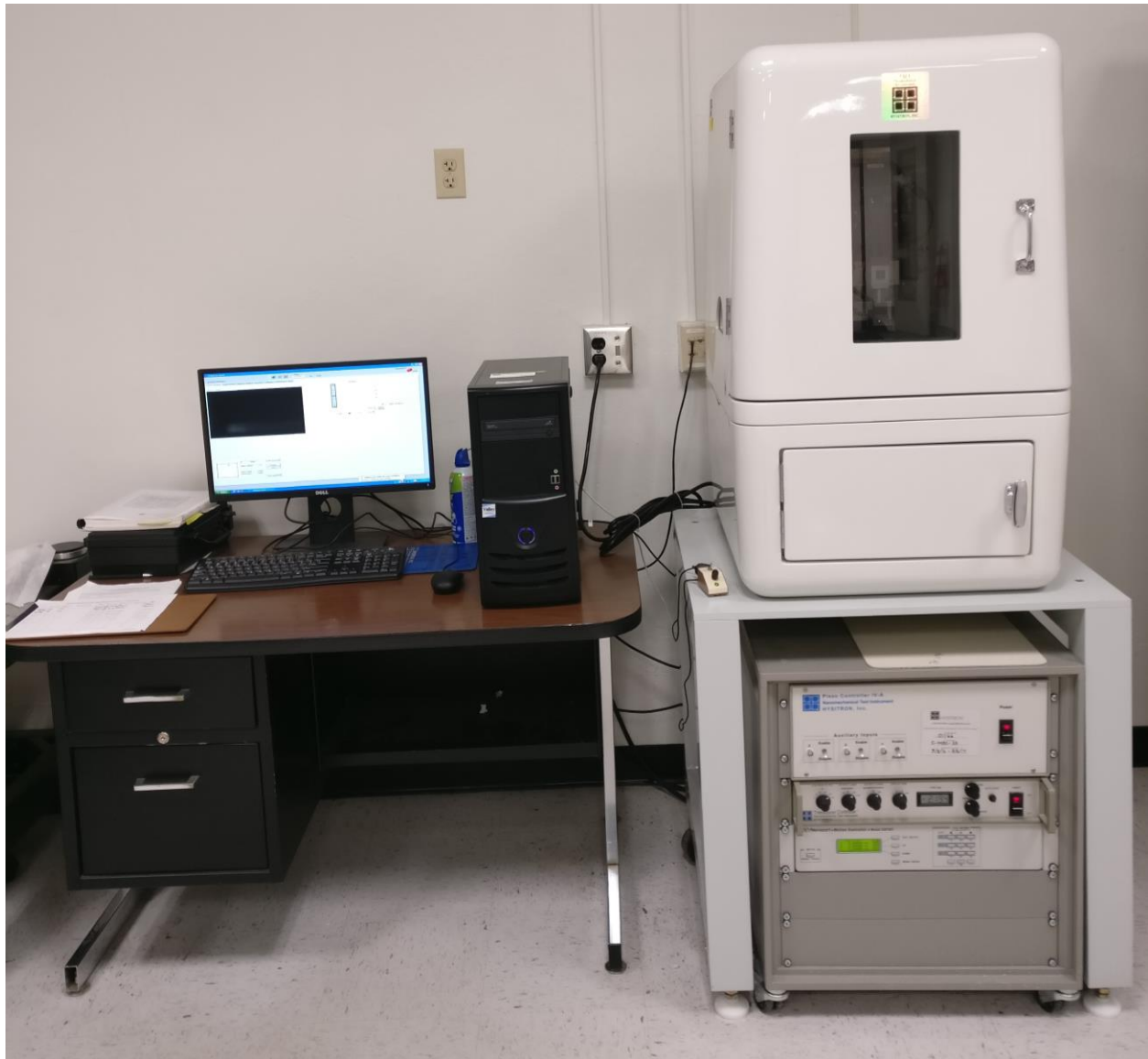
Fig. 3.3: Hysitron Ubi-1 Nanoindenter used in this project.
