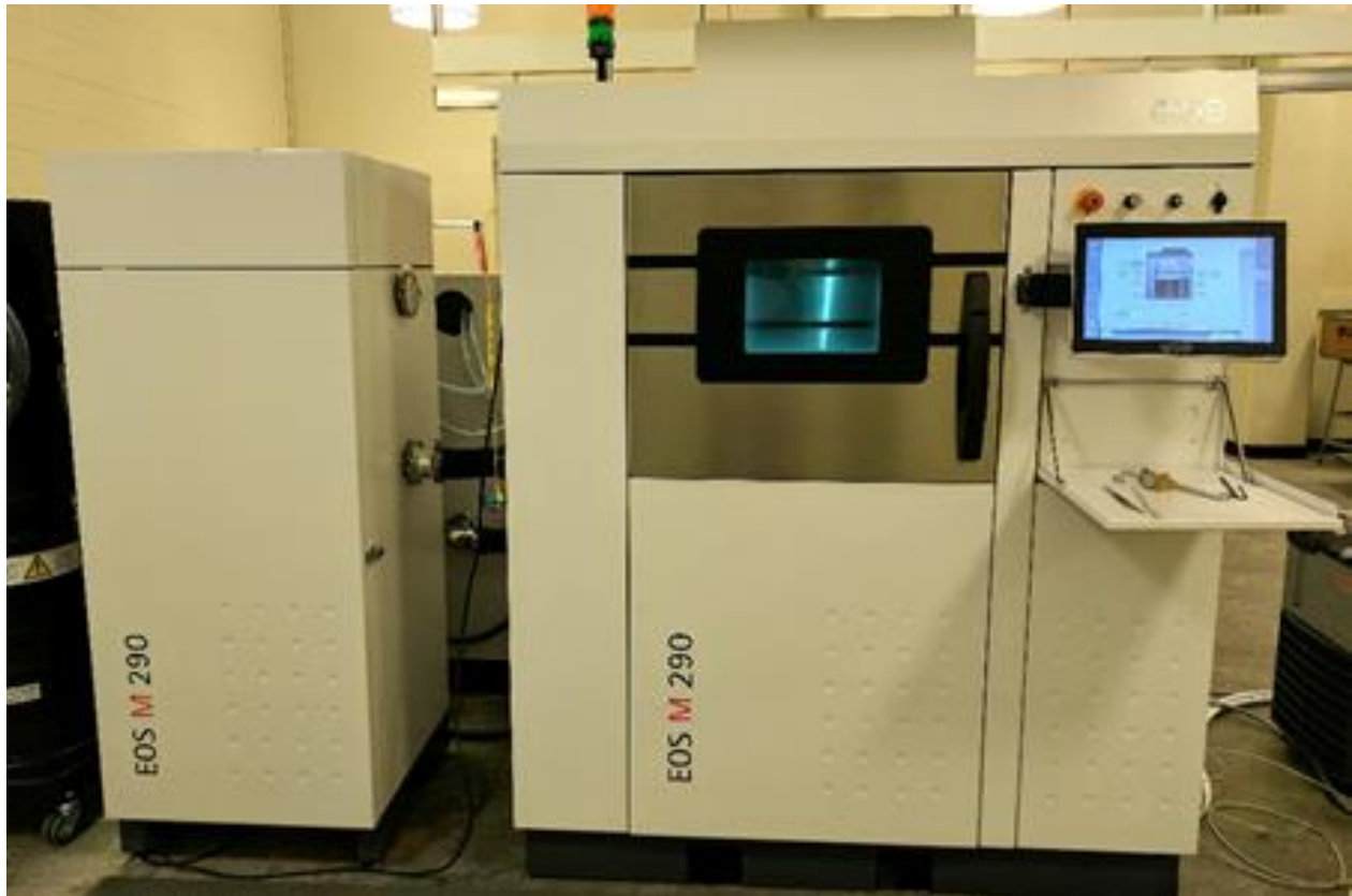
Fig. 3.2: EOS 290 3D printer used in this research to print the samples.
