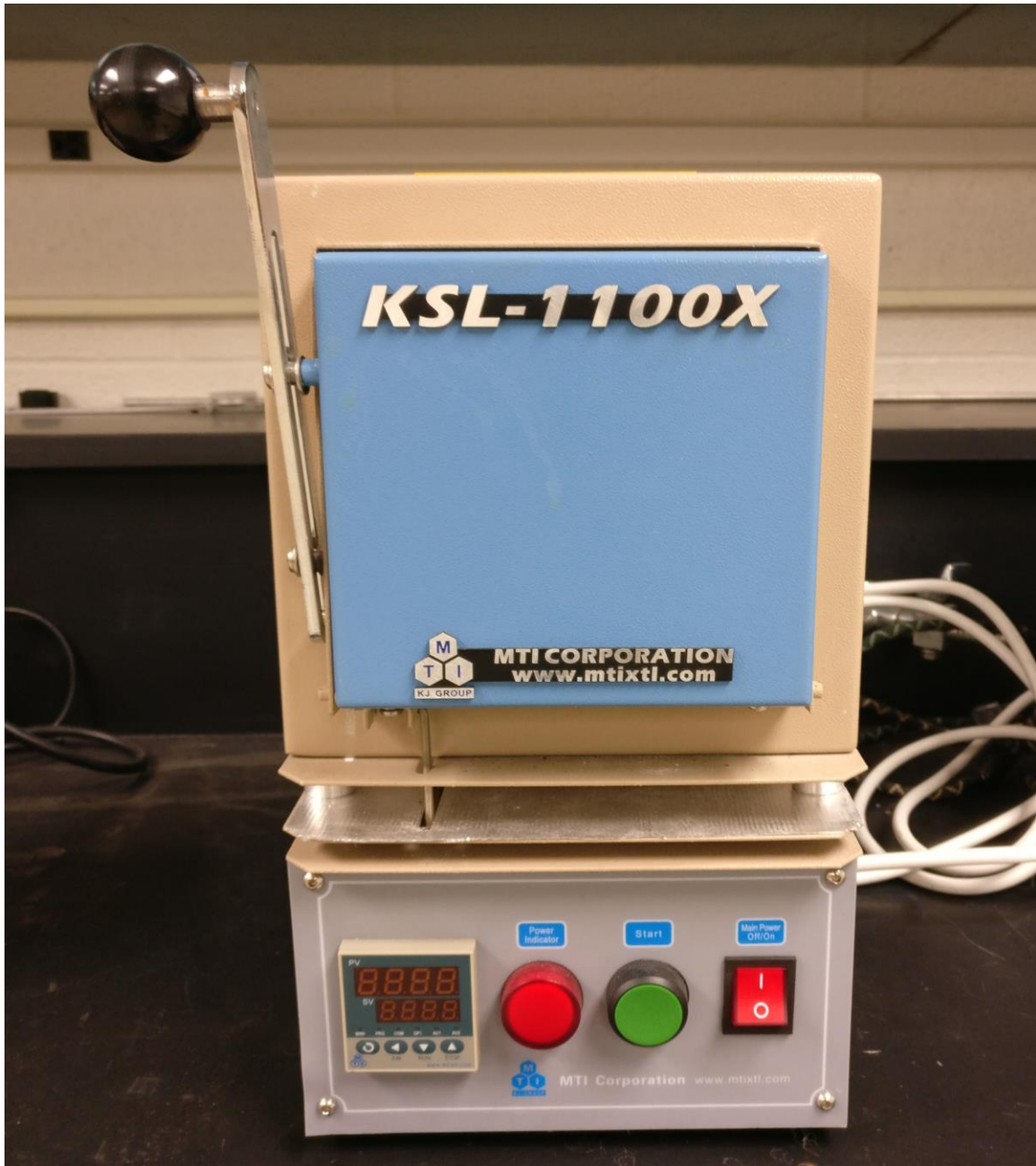
Fig. 3.13: KSL-1100X furnace used to perform heat treatment in this study.
