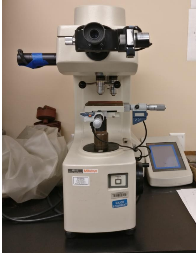
Fig. 3.14: HM 112 Mitutoyo used to test micro-hardness in this project.
