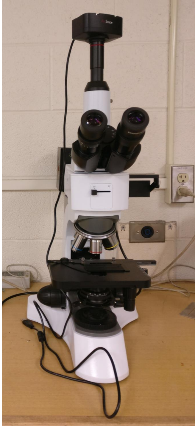
Fig. 3.6: Optical Microscope (MM500T) employed in this study for microstructural assessments.
