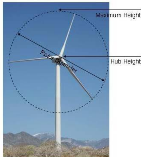
Figure 3. Geometrical parameters of horizontal axis wind turbines [4]
