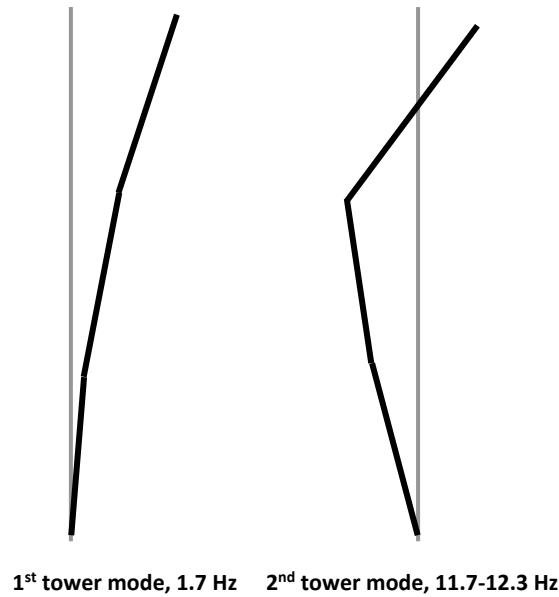
Figure 23. Observed 1 st and 2 nd mode shapes [36]
