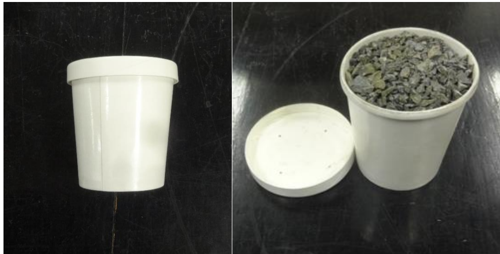
Figure 11A and 11B. The pint-sized paper storage containers used to store the rock fragments after sample preparation.
