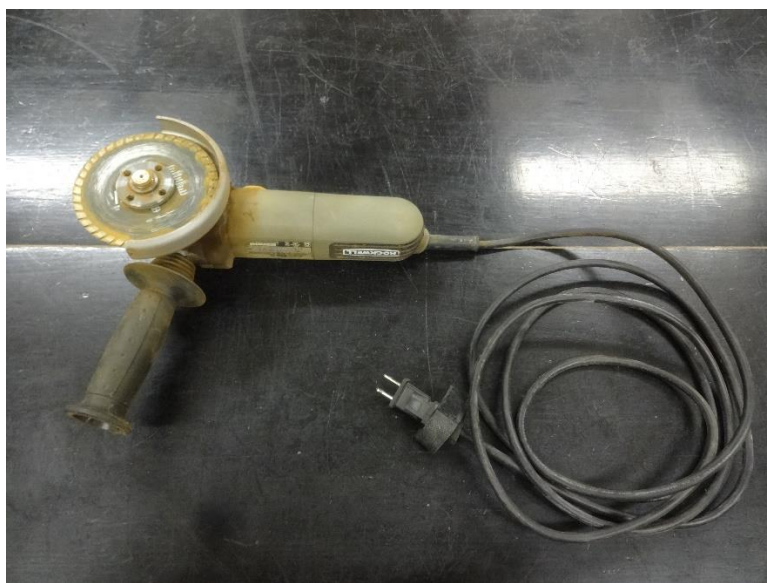
Figure 9. Cut-off saw used for cutting specifically igneous rocks.
