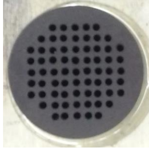
Fig. 3.1.1 Sintered ferrite sample with holes drilled.
