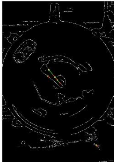
Figure 4.5: Phase angle of the unbalanced flywheel.
