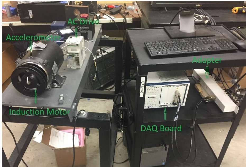
Figure 3.1: The experiment setup for obtaining vibration data.
