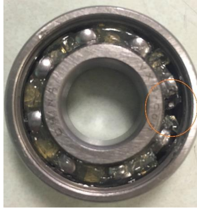
Figure 3.11: The damaged bearing
