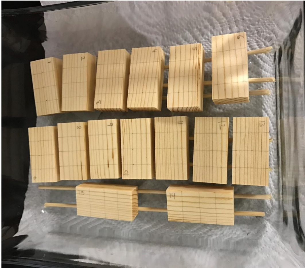
Figure C. 1. Ponderosa pine wood samples ( 5.0 \times 2.5 \times 1.5 \text{ cm}^3 ) dipped in the radiolabeled Woodlife solution and placed on wooden skewers to dry for 24 hours.
