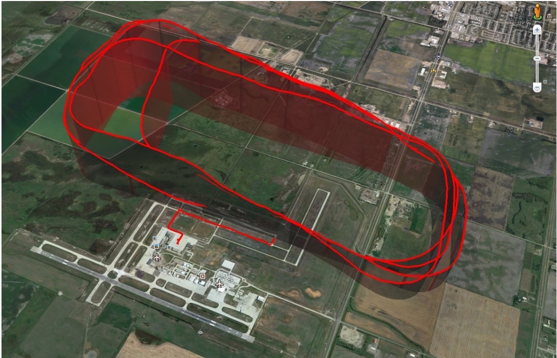
Figure 12: Example of using a KML file to visualize a flight path in Google Earth . This flight visualization is an example of a student flight that has multiple approach phases.
