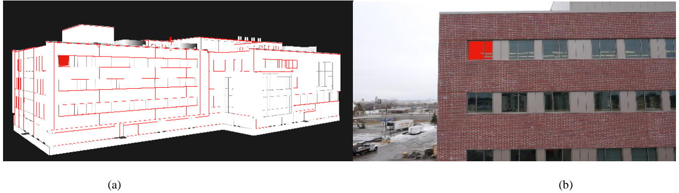
Figure 2.2: Image registration to 3D CAD model (a) Selected four corners of the window shown in red from CAD model (b) Corresponding four corners selected in the first keyframe of the red marked window.
