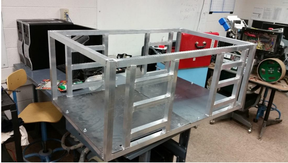
Figure 67 - Manufactured Frame and Steel Plates
