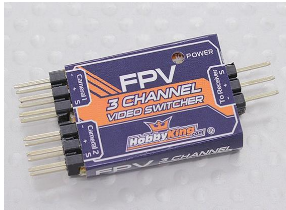
Figure 90 - 3 Channel Video Switch (Hobbyking, n.d.)
