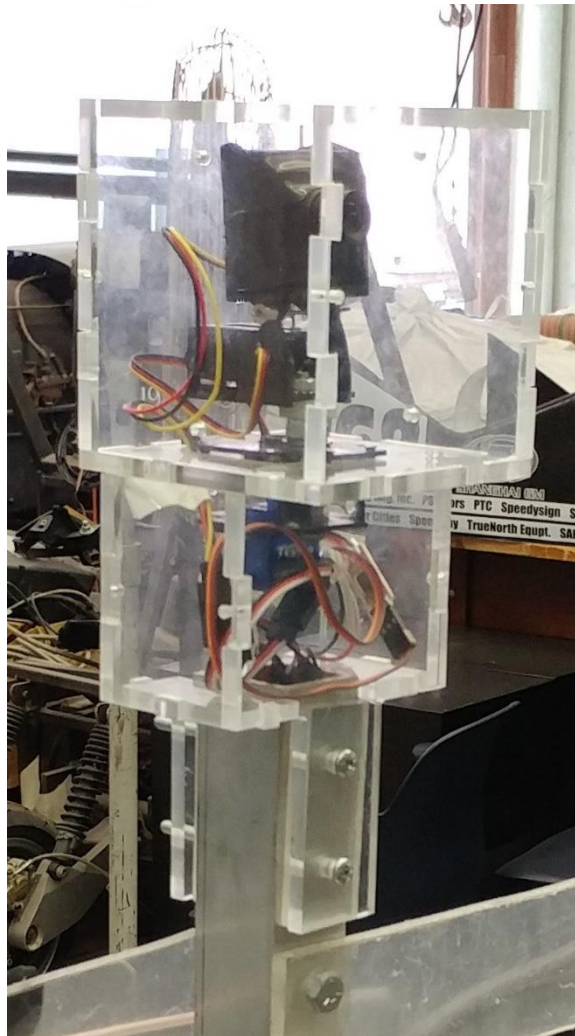
Figure 89 - Completed Rover Camera Housing
