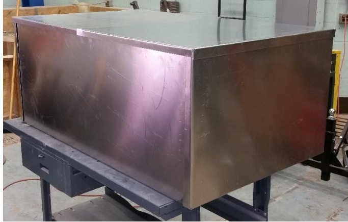
Figure 69 – Frame with Aluminum Panels
