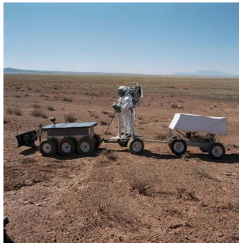
Figure 8 - ET hauling the Chariot and Science Trailer (Ross, Kosmo, & Janoiko, 2010)
