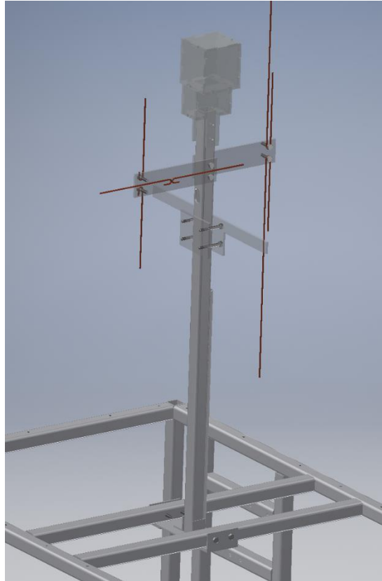
Figure 68 - Antenna and Camera Boom
