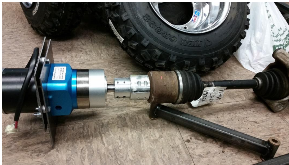
Figure 54 - Completed Drivetrain Assembly
