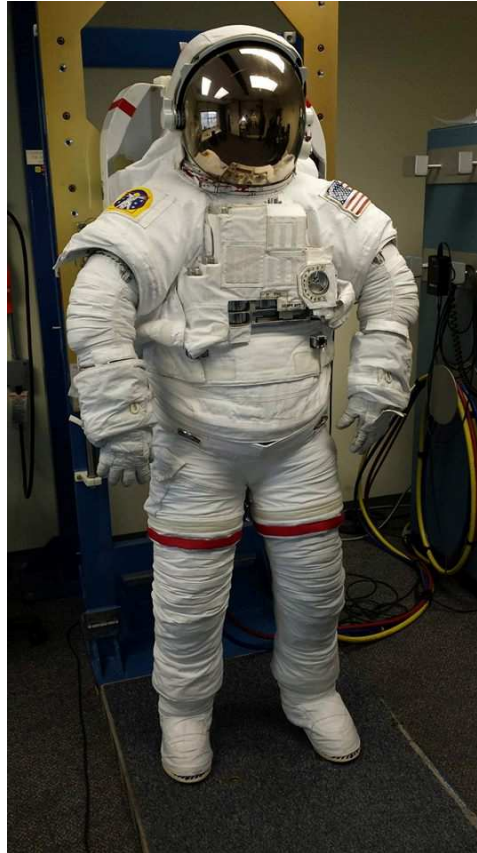
Figure 12. Extravehicular Mobility Unit used for the Shuttle and ISS programs. Photo: Author
