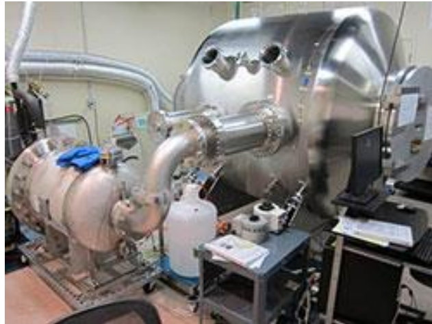
Figure 44. Paragon SDC EHF hypobaric testing chamber.
