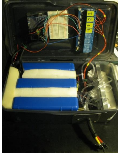
Figure 30. Wiring the controller, relays and pumps into enclosure.
