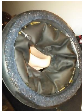
Figure 59. Gel seal ring on prototype transitional seal (note Schrader valve for ring inflation.).
