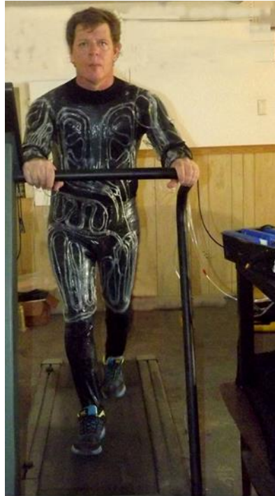
Figure 43. Cooling system testing on treadmill.
