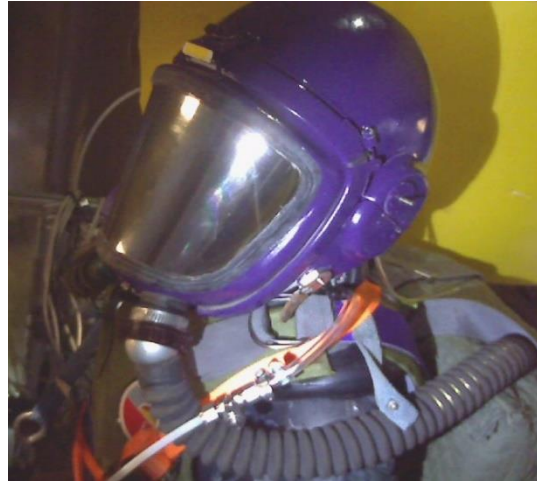
Figure 58. Transitional neck seal in EHF Hypobaric chamber as captured from video camera during depress cycle.
