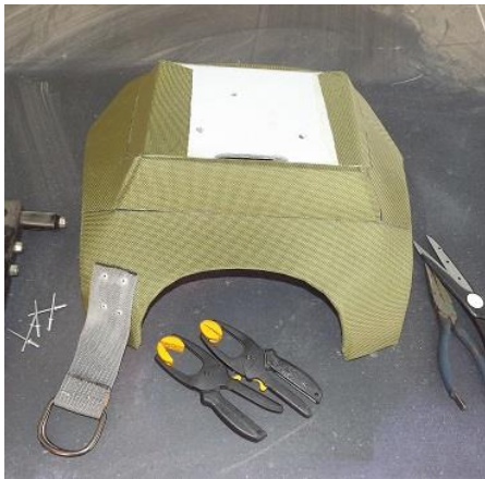
Figure 15. Hard torso ballistic Nylon coating.
