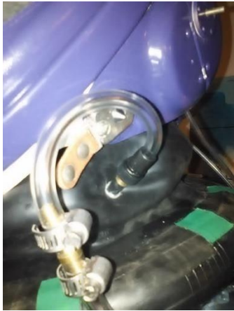
Figure 57. Helmet internal pressure monitoring line detail.
