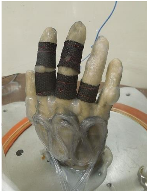
Figure 52. Partially completed glove liner in hard vacuum.
