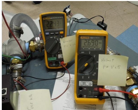
Figure 50. Multi-meters for hypobaric chamber and helmet pressure sensor readings.
