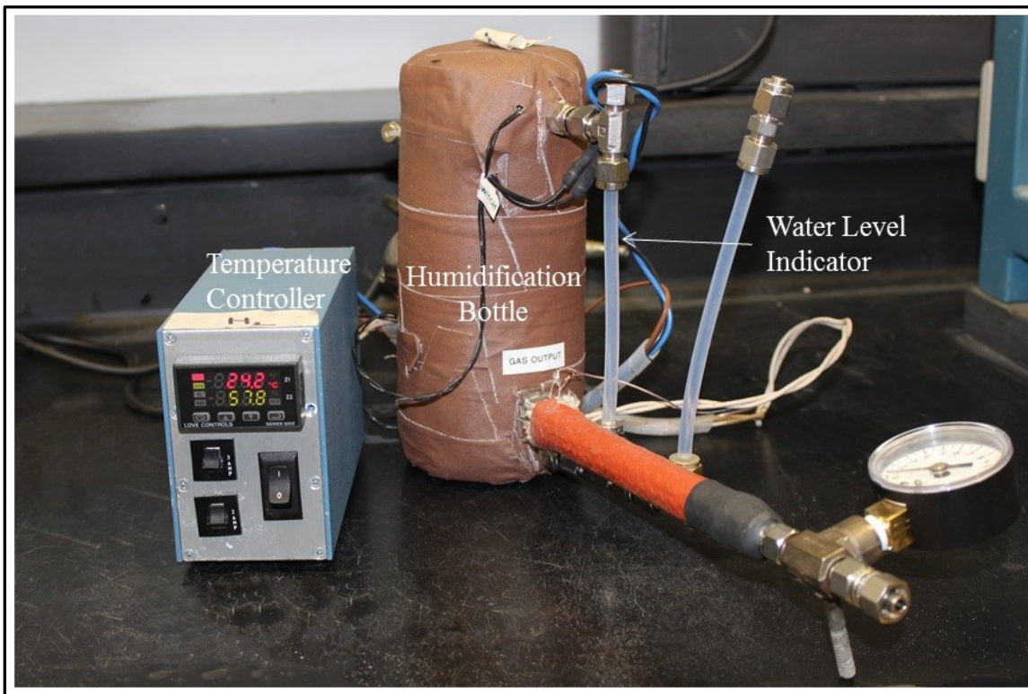
Figure 4-14 Humidification System used for reactants humidification
