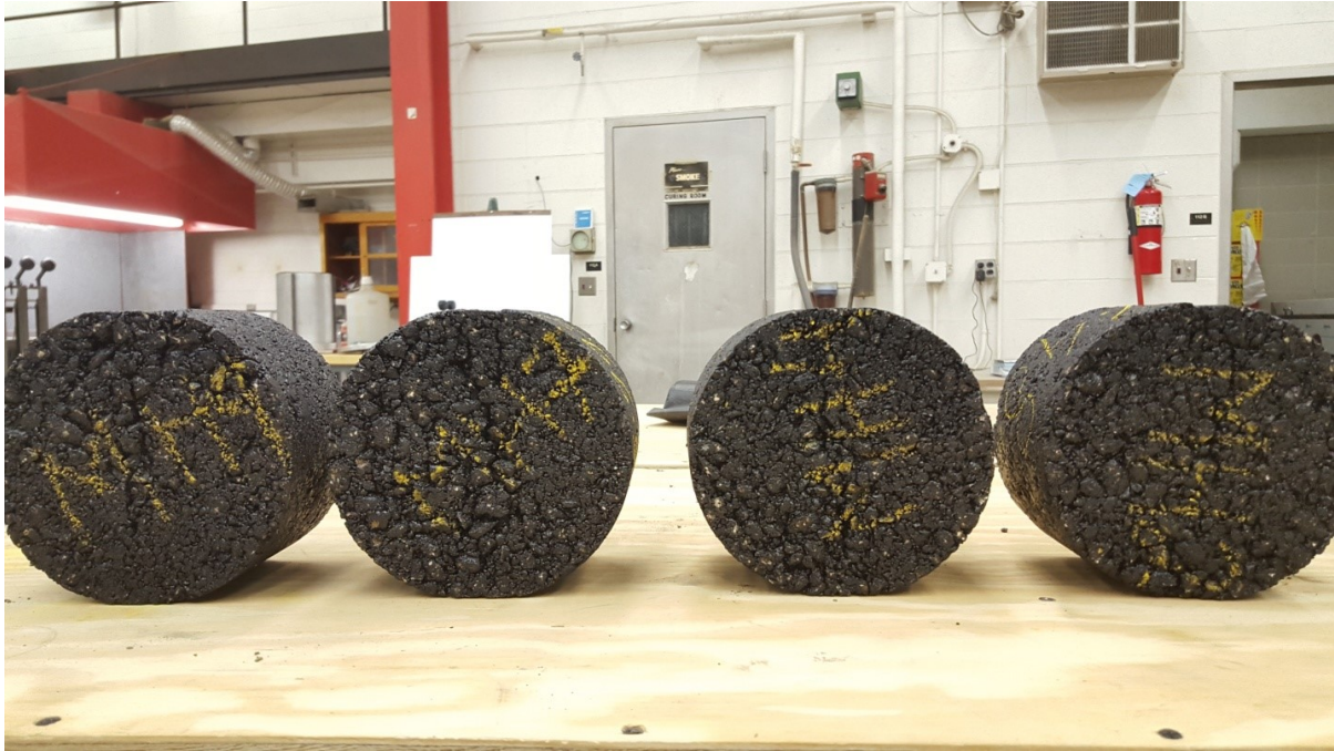
Figure 15 Visible Cracking in the dry Non-Conventional specimens after Modified Lottman Test
