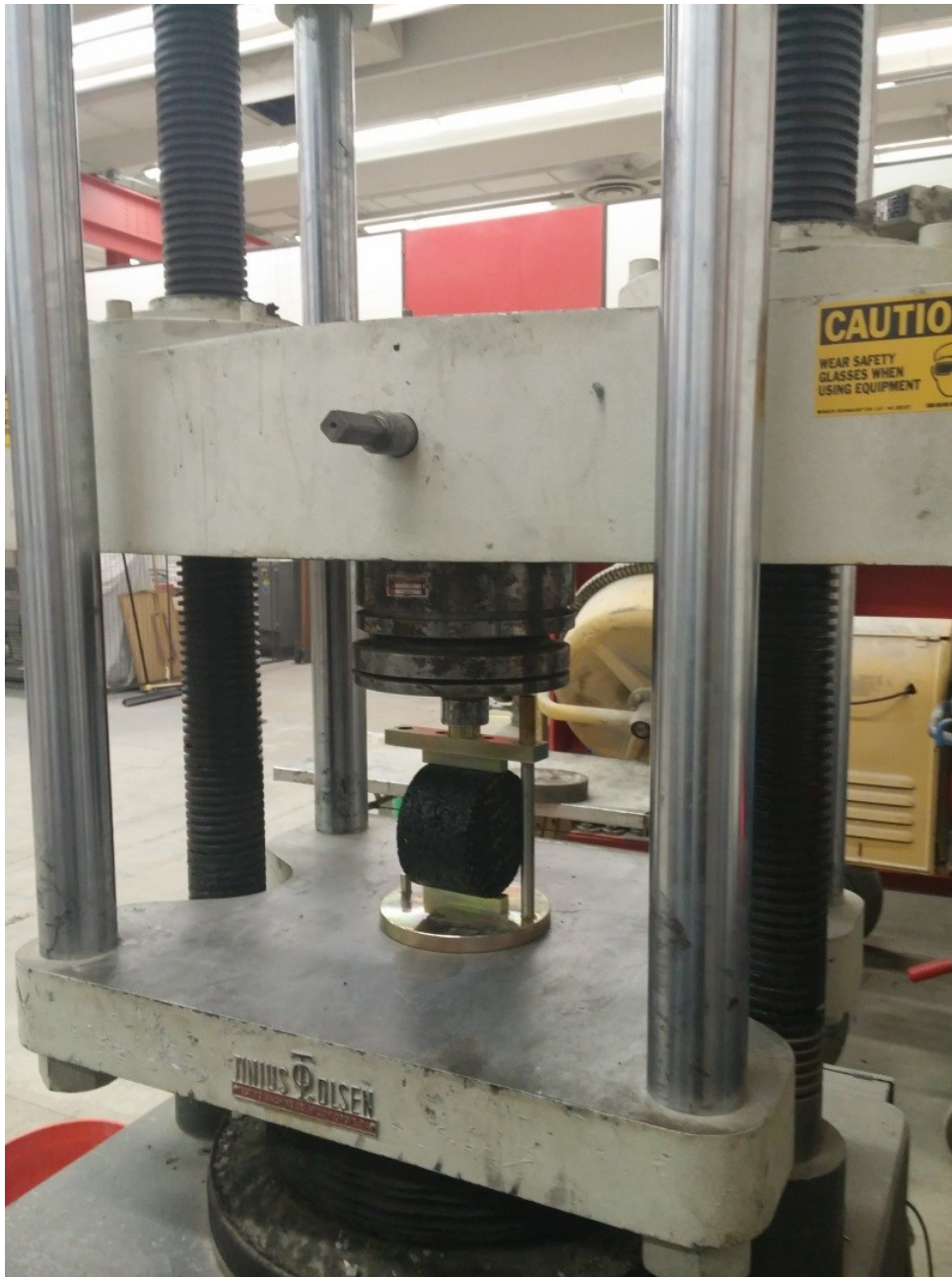
Figure 6 Specimen placement between bearing plates
