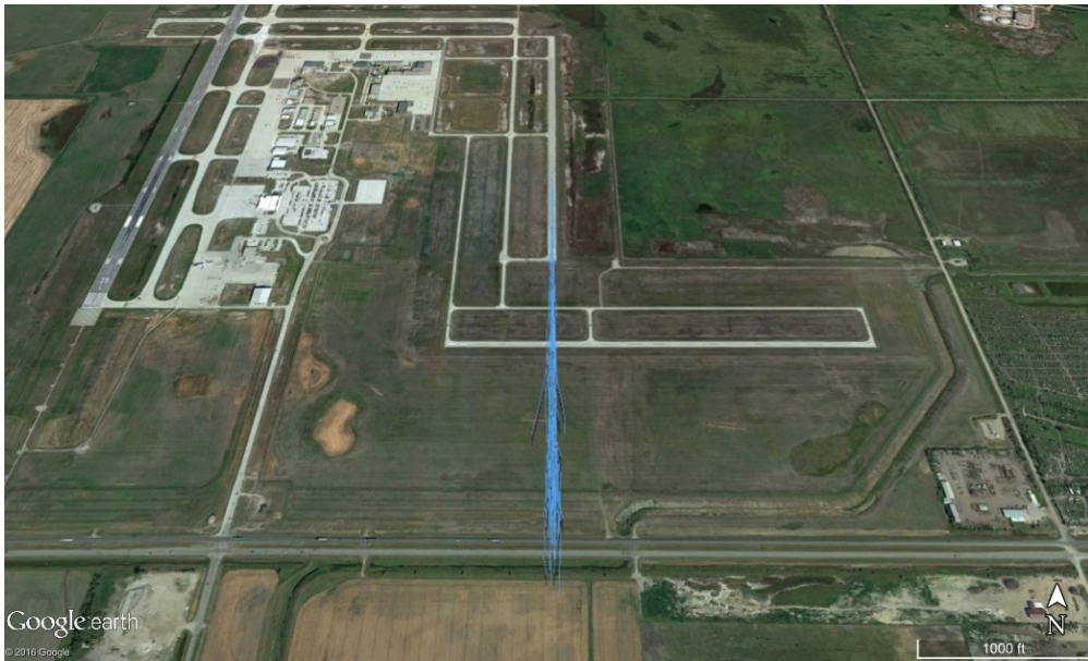
Figure 25: Cluster 2 - Aerial view of approaches that were on average 7 knots faster than UND's SOP; however they were stabilized.
