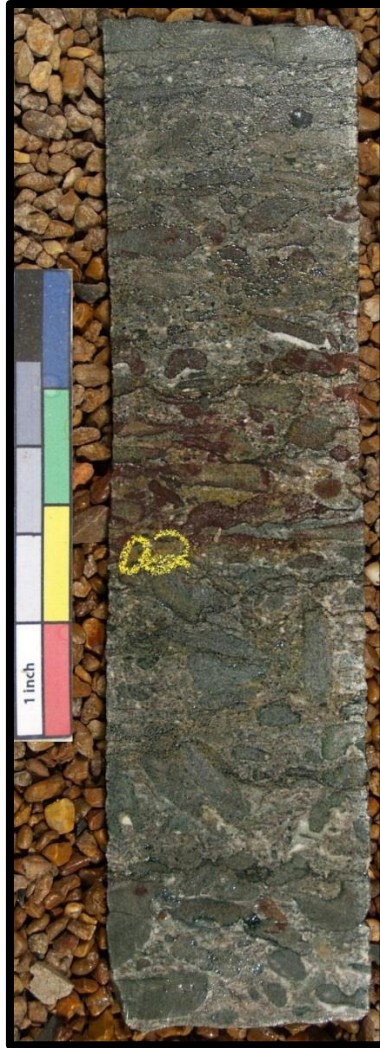
Figure 14. A photograph of core from NDGS #6624 at a depth of 9,302'. Displaying a conglomerate from above the contact with the Precambrian gneiss. It is dominated by glauconitic quartz arenite.
