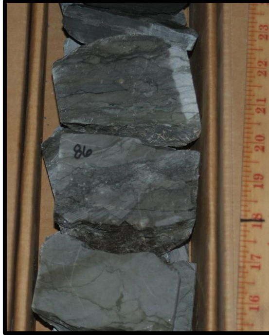
Figure 17. A photograph of core from NDGS #291 at a depth of 13,286'. An example of the burrow-mottled limestone found in Member C, contain siliciclastic mudstone laminae and intraclastic wackestone and packstone.
