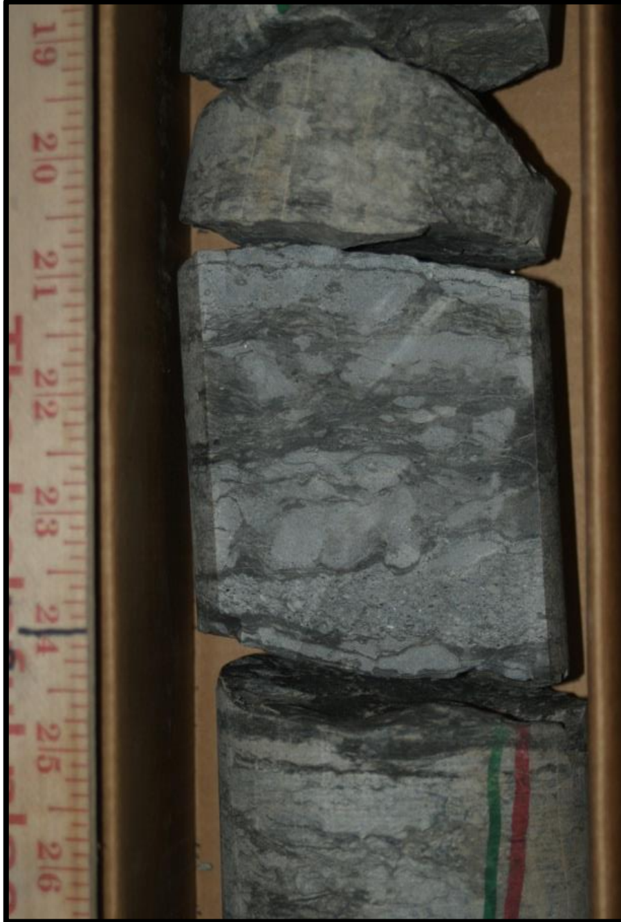
Figure 19. A photograph of core from NDGS #291 at a depth of 13,193'. An example of the gradation upwards to a fine-grained, siliciclastic burrow-mottled mudstone. The ruler is in inches.
