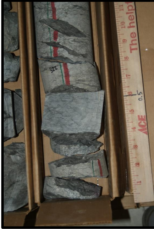
Figure 16. A photograph of core from NDGS #291 at a depth of 13,322'. Characteristic light gray, packstone to grainstone limestone occurring in Member C.
