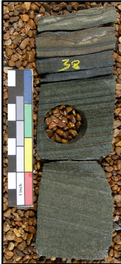
Figure 15. A photograph of core from NDGS #6624 at a depth of 9,238'. Displaying planar laminated glauconitic siltstone, with minor cross beds.
