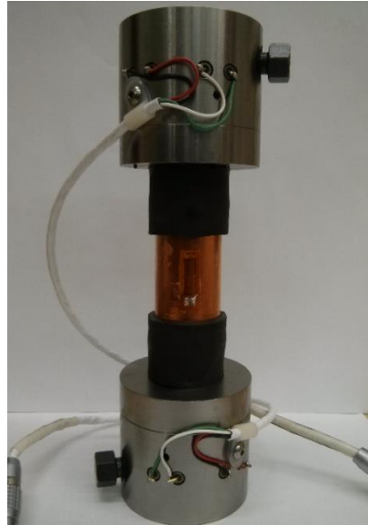
Figure 3.18 Core holder with an instrumented Bakken sample that is jacketed and positioned between velocity transducers with strain gages attached
