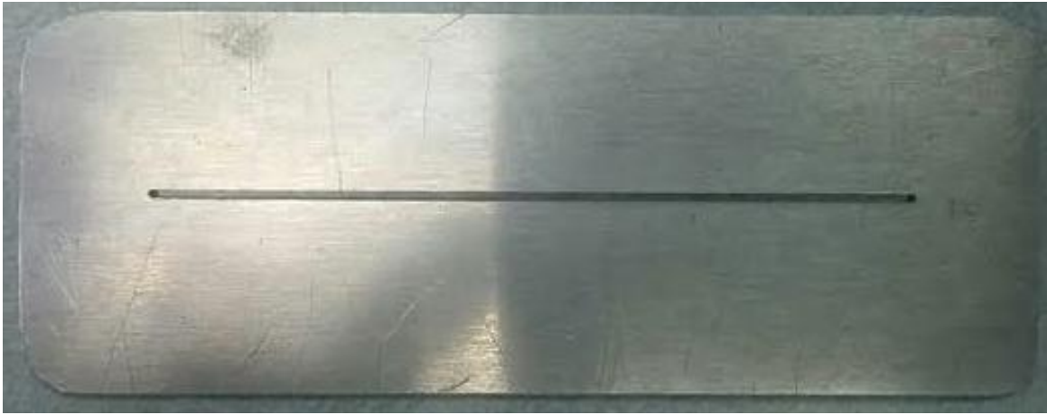
Figure 37 Image of middle test section used in the porous medium testing.
