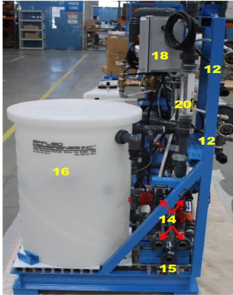
Figure 4.5.4.3. RO pilot system PW-4XM-14A-116 side view.
