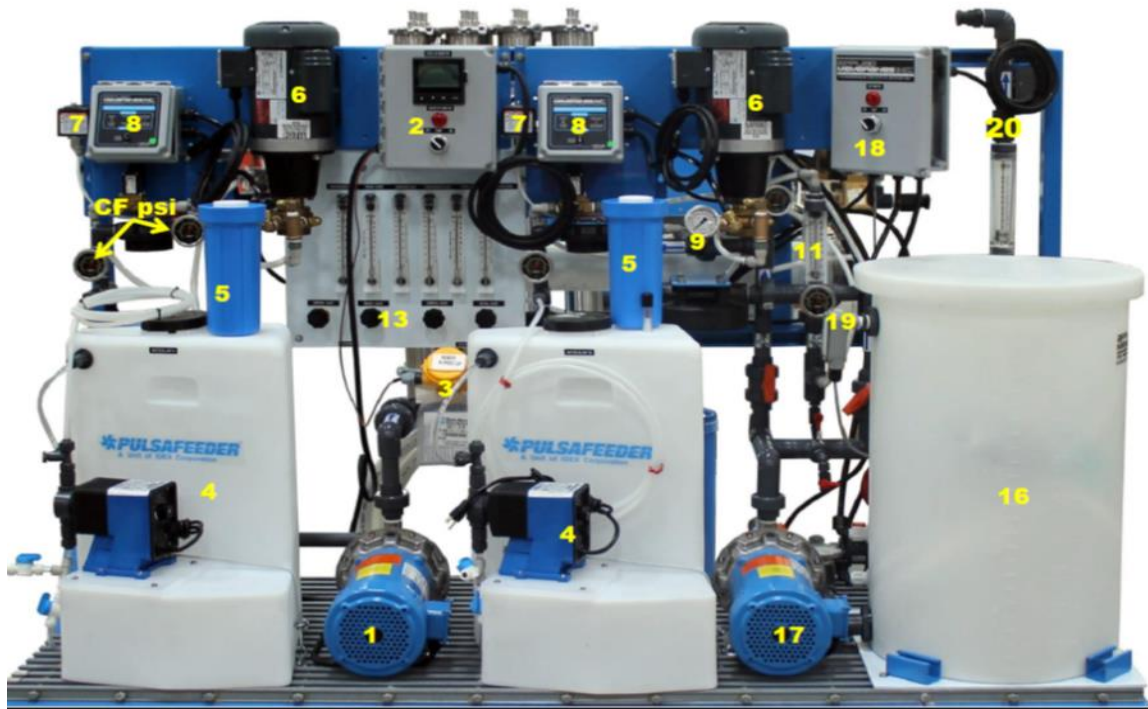
Figure 4.5.4.1. RO pilot system PW-4XM-14A-116 front view.
