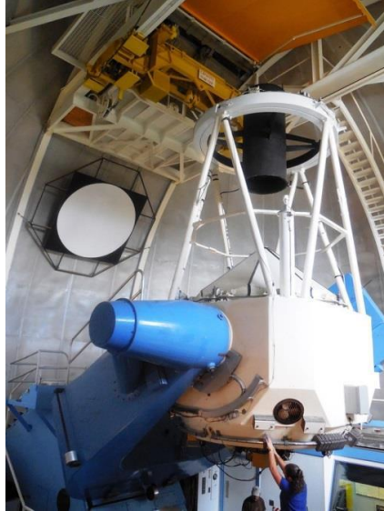
Fig. 17 – The NOAA 2.1-meter Telescope at Kitt Peak National Observatory: pictured here with a KPNO staff member installing lead counterweights to balance the telescope. Note black secondary mirror housing above and white flat screen in background used in calibration.
