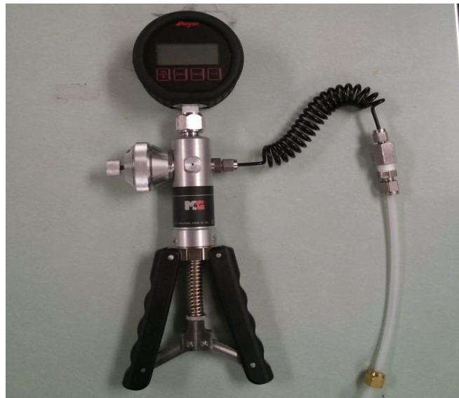
Figure 3.15: Ametek hand pump attached to Dwyer digital gage
