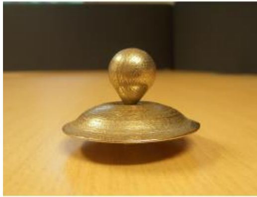
Figure 8. 3D printed volcano smoke antenna [45].
