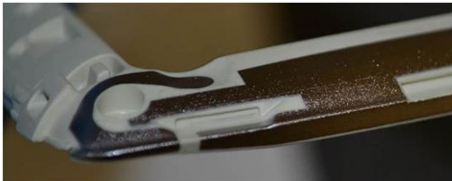
Figure 6. Antenna printed with Aerosol Jet direct write process [32].
