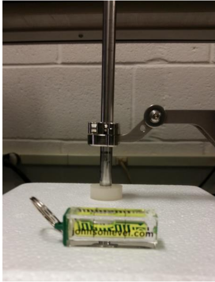
Figure 23. 85070E Agilent performance probe and a material under test.
