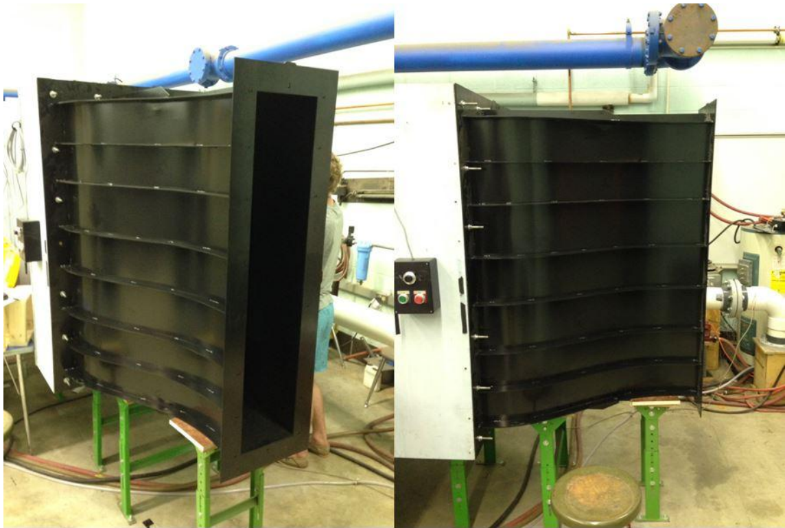
Figure 22. Installed new LT nozzle.
