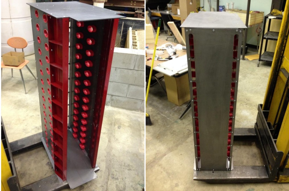
Figure 31. Photos of completed turbulence generator mock liner.
