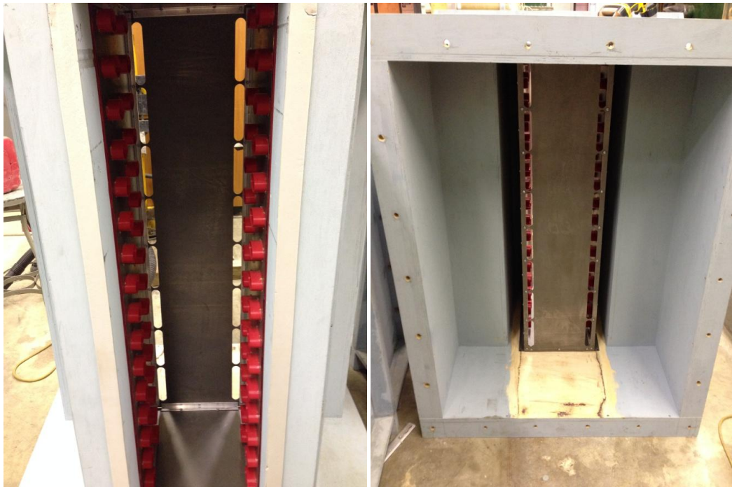
Figure 32. Photos of fully completed turbulence generator.
