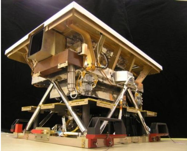
Figure 1-23. VIR built by Italian Space Agency ASI and National Institute for Astrophysics INAF; hyperspectral spectrometer; wavelength range: 0.25 to 5 \mu\text{m} ; from: Selex Galileo, INAF, and ASI.
