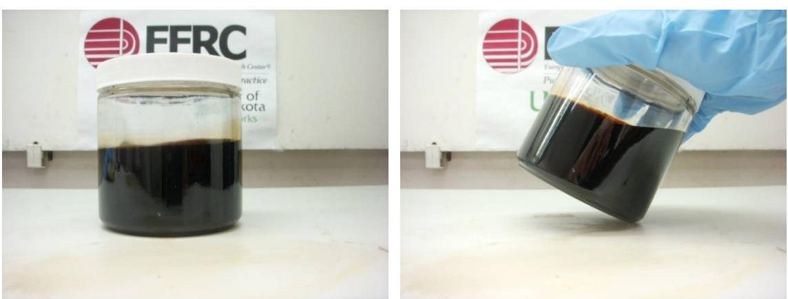
(a) (b) Figure 7-60. Hi-pour fuel oil – biocrude blend, cooled from 170°F to 75°F. (a) shows the blend sitting flat, and (b) shows the blend tilted at an angle.
