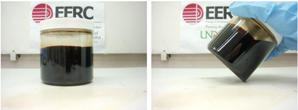
Figure 7-66. Lo-pour fuel oil – biodiesel blend, cooled from 170°F to 75°F. (a) shows the blend sitting flat, and (b) shows the blend tilted at an angle.
