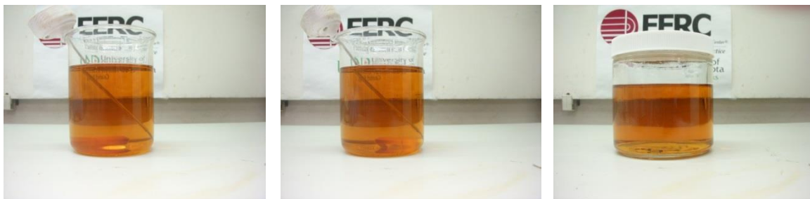
Figure 7-35. Crude jatropha oil – biodiesel blend, mixed and held at 170°F. (a) immediately after five minutes of stirring, (b) 25 minutes after stirring, (c) six days after stirring.
