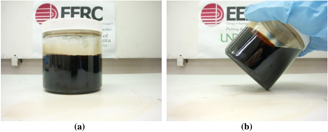
Figure 7-67. Lo-pour fuel oil – ultra-low sulfur diesel blend, cooled from 170°F to 75°F. (a) shows the blend sitting flat, and (b) shows the blend tilted at an angle.
