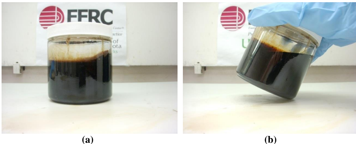
Figure 7-58. Hi-pour fuel oil – crude palm oil blend, cooled from 170°F to 75°F. (a) shows the blend sitting flat, and (b) shows the blend tilted at an angle.
