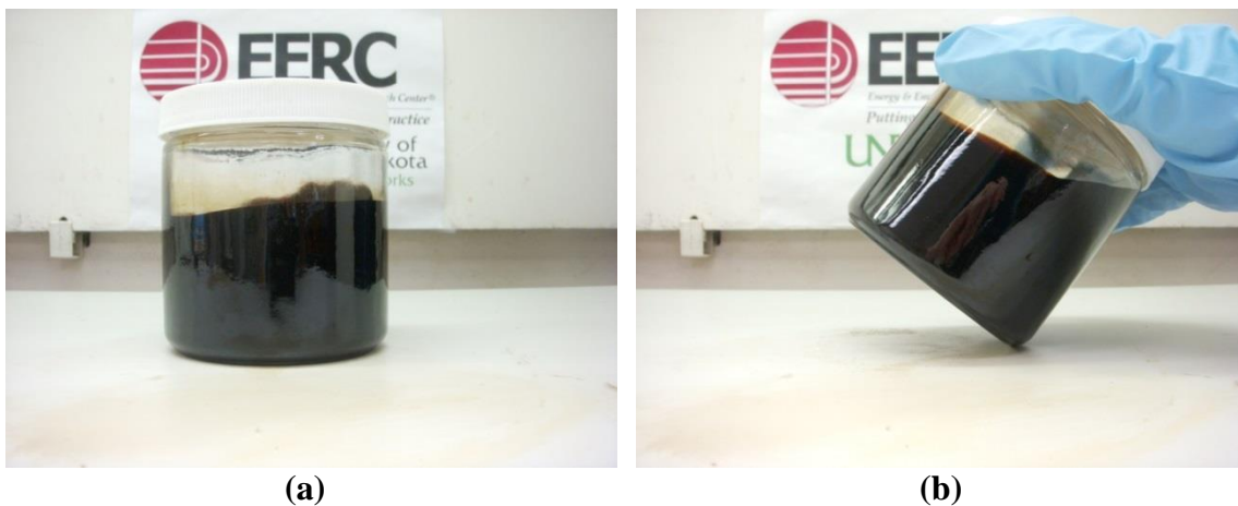
Figure 7-79. Hi-pour fuel oil – biocrude blend, cooled from 220°F to 75°F. (a) shows the blend sitting flat, and (b) shows the blend tilted at an angle.
