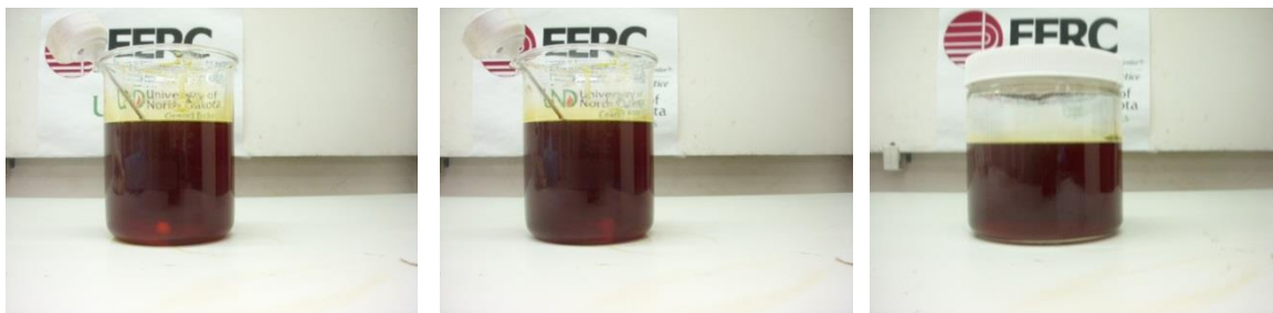
Figure 7-31. Crude palm oil – biocrude blend, mixed and held at 170°F. (a) immediately after five minutes of stirring, (b) 25 minutes after stirring, (c) five days after stirring.
