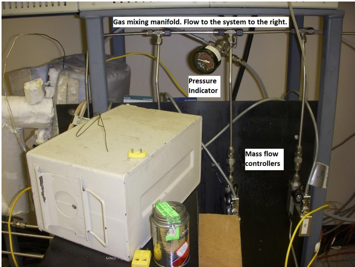
Figure 3-8. Mass flow controllers, pressure indicator, and stainless steel manifold for mixing syngas.
