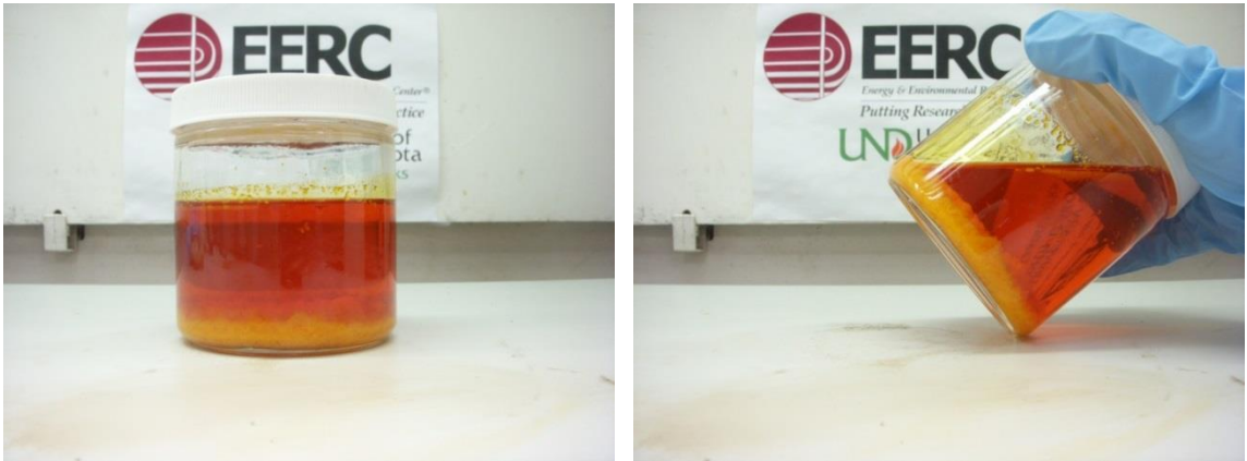
(a) (b) Figure 7-71. Crude palm oil – ultra-low sulfur diesel blend, cooled from 170°F to 75°F. (a) shows the blend sitting flat, and (b) shows the blend tilted at an angle.
