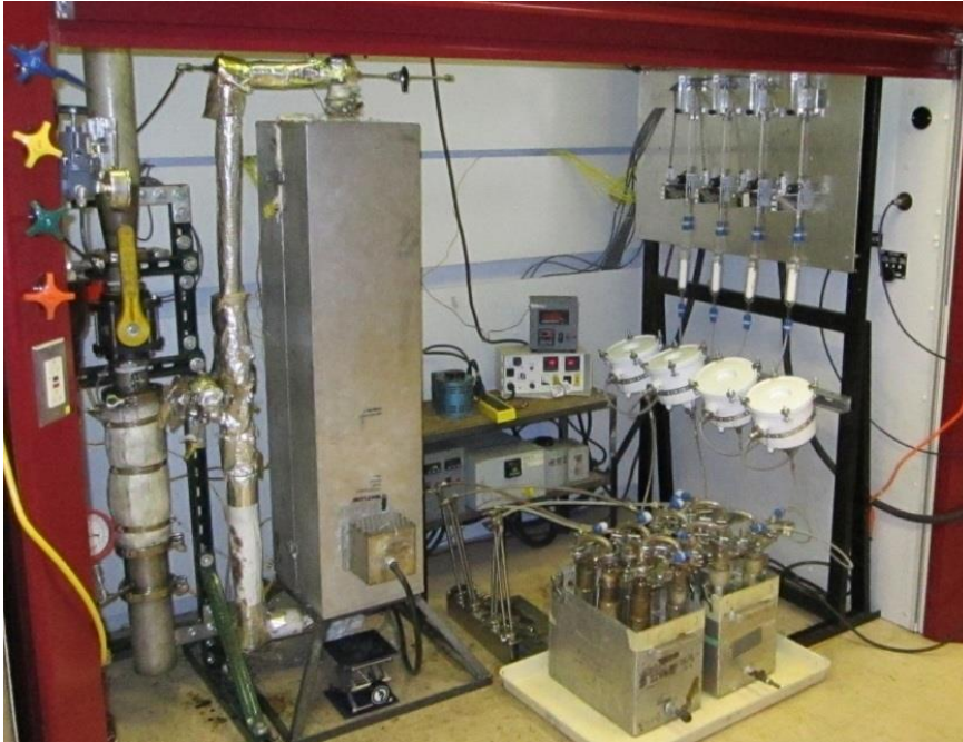
Figure 3-4. Laboratory-scale updraft gasifier and tar cracker.
