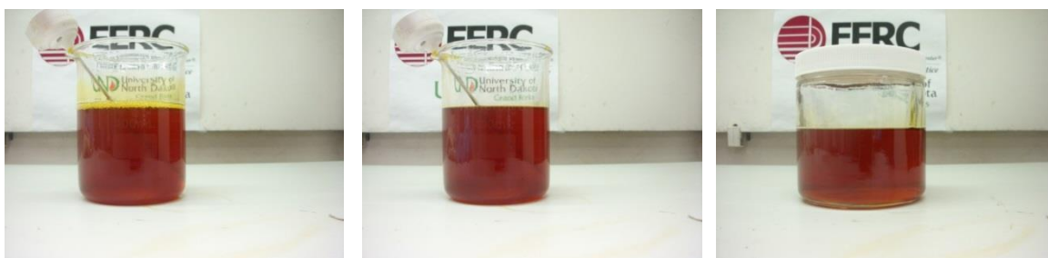
Figure 7-32. Crude palm oil – biodiesel blend, mixed and held at 170°F. (a) immediately after five minutes of stirring, (b) 25 minutes after stirring, (c) five days after stirring.
