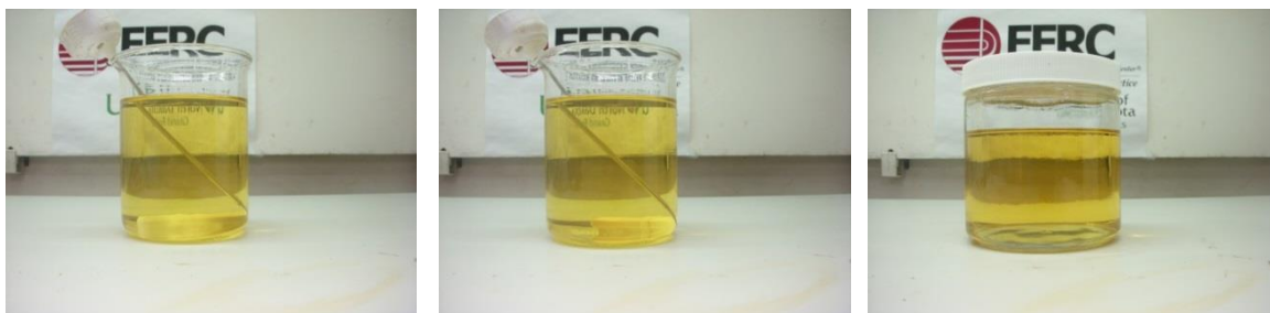
Figure 7-36. Crude jatropha oil – ultra-low sulfur diesel blend, mixed and held at 170°F. (a) immediately after five minutes of stirring, (b) 25 minutes after stirring, (c) six days after stirring.
