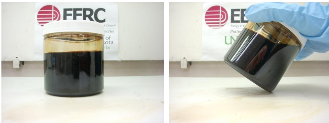
Figure 7-78. Hi-pour fuel oil – crude jatropha oil blend, cooled from 220°F to 75°F. (a) shows the blend sitting flat, and (b) shows the blend tilted at an angle.
