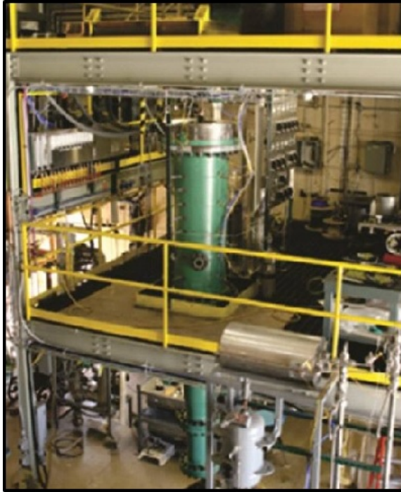
Figure 2.1: Photograph of the EERC Entrained-Flow Gasifier used.
