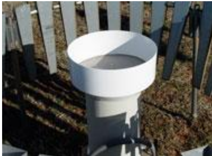
Figure 5. An unheated tipping bucket with alter shield that is used for OK MESONET precipitation observations.
