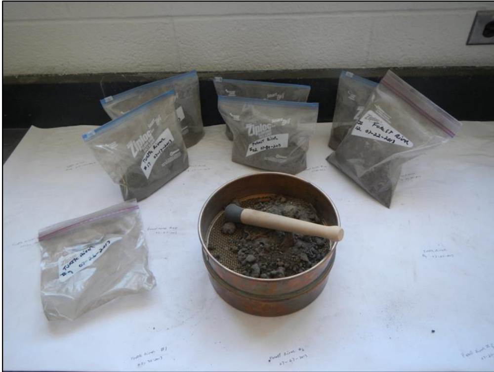
Figure 10. Soil sieve to \leq 2 mm.
