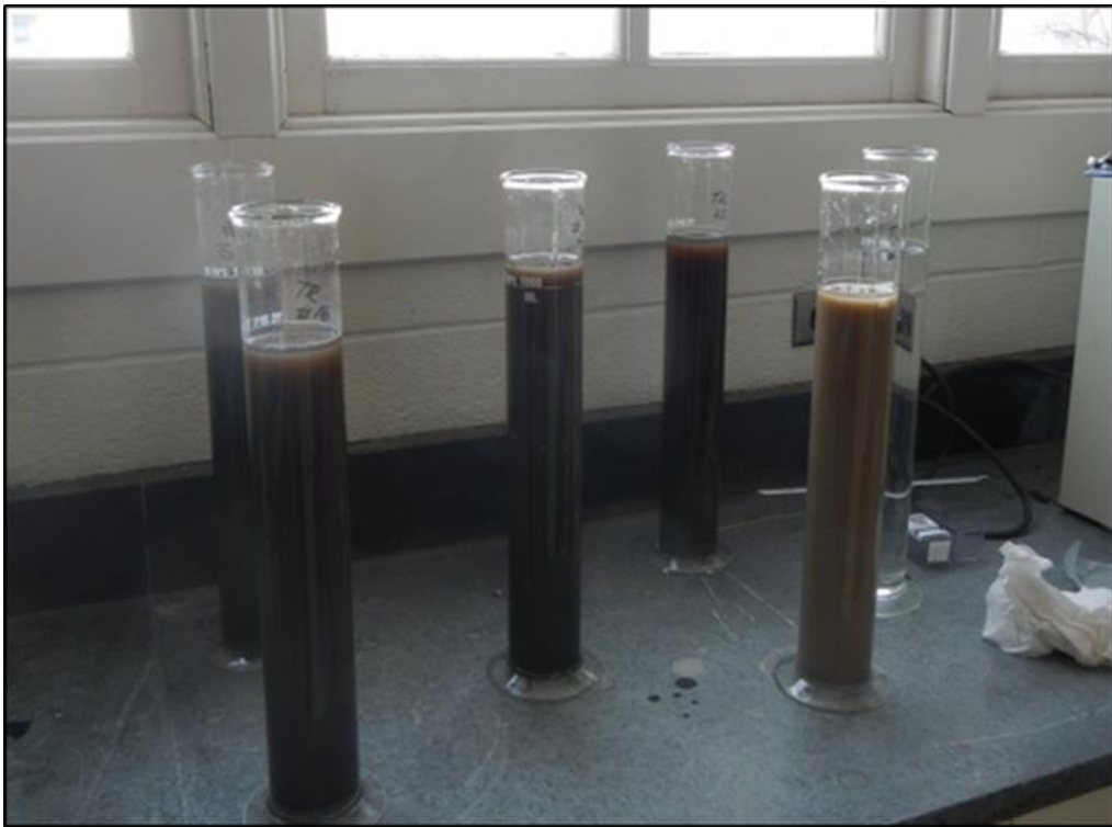
Figure 11. Separates analysis using the hydrometer method.
