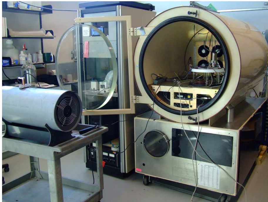
Fig 5. The Low Pressure Test Bed and Wind Tunnel in Preparation Stage for Forced Convection Testing.
