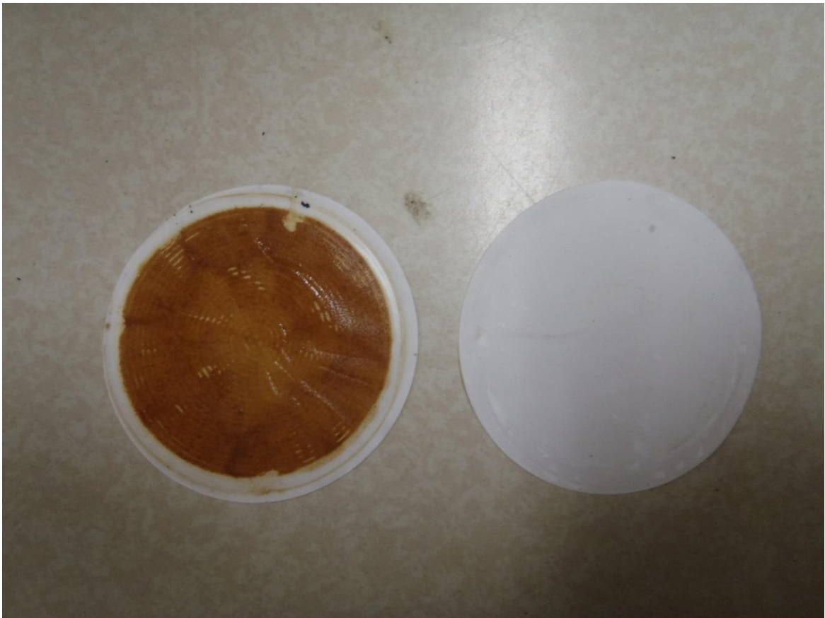
Figure 12: Picture of 0.45 micron filters after filtration. Left filter is from a turbid sample taken from the sand layer at 45 cm and the right filter is from a regular 45 cm sample.
