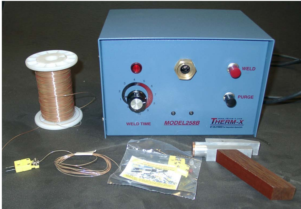
Figure 39. Thermocouple welder, materials, and completed thermocouple.
