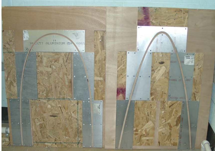
Figure 33. Large and small cylindrical leading edge test section router jigs.
