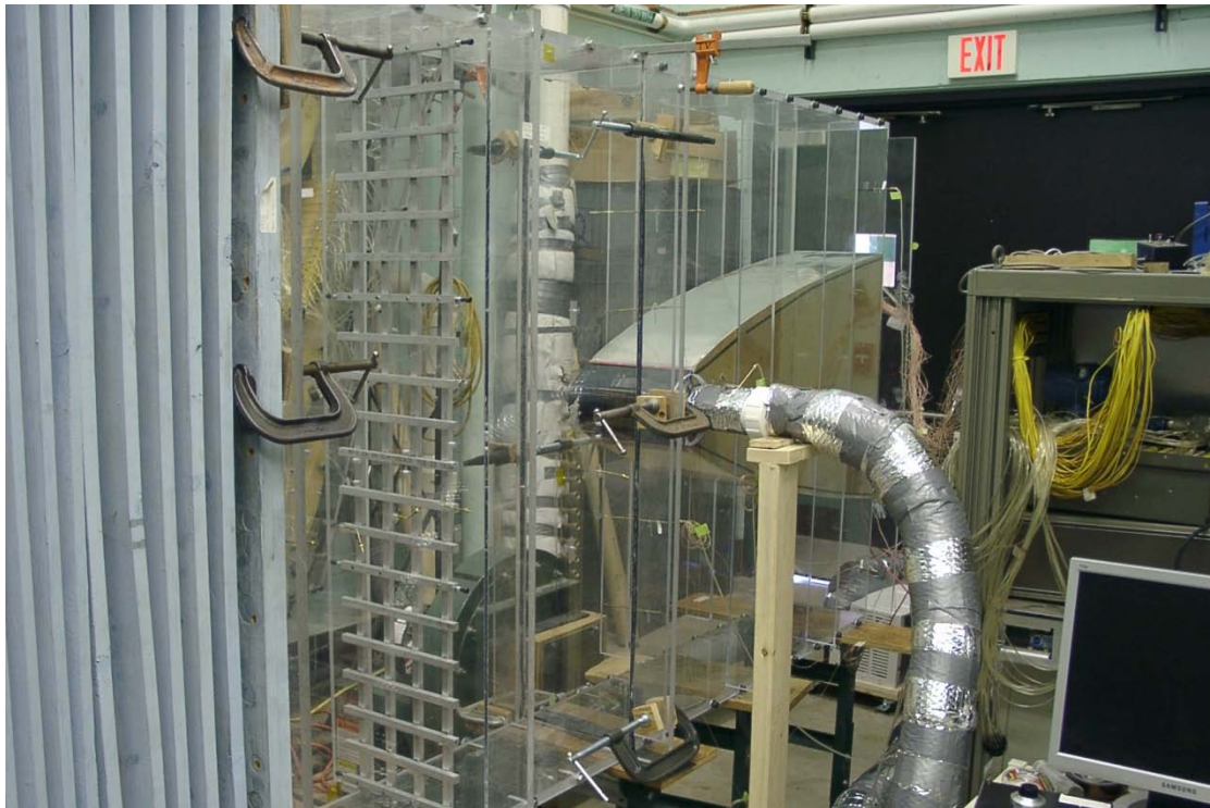
Figure 46. Small cylindrical test section, large grid.
