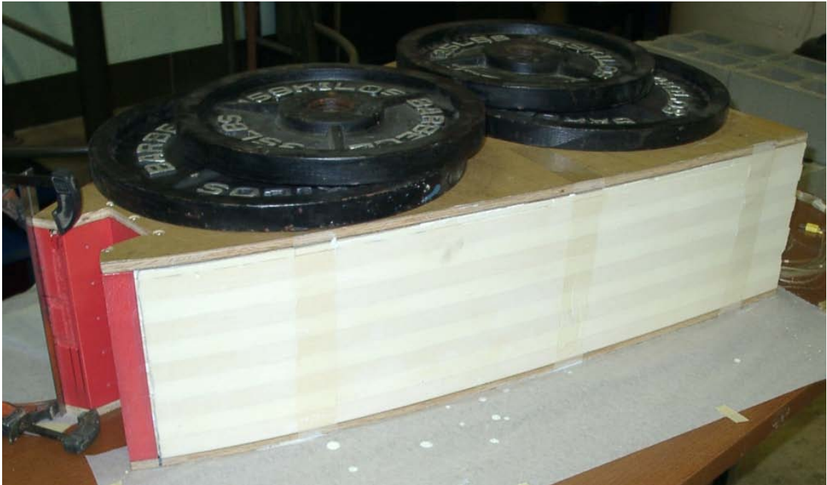
Figure 36. Small test section with mounting bracket attached and weights applied.
