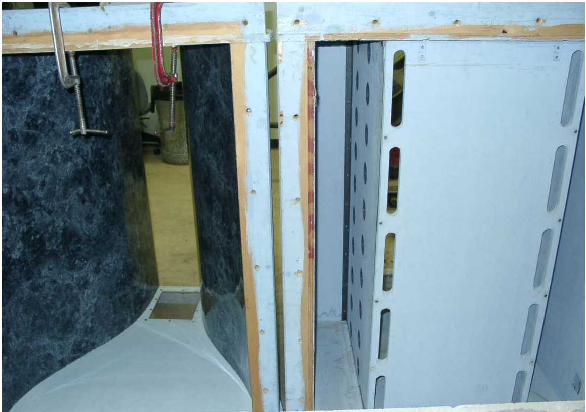
Figure 15. Laminar flow nozzle and mock aero-combustor, rear view.
