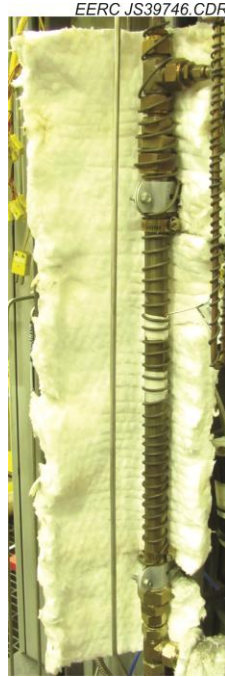
Figure 3.3. SS1 Membrane Mounts and Heat Trace.
