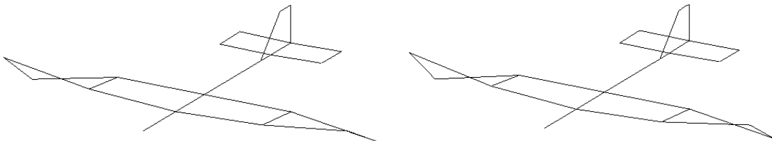
Figure 71. Mode shape corresponding to a frequency of 28.1 Hz for WH (left) and 28.9 Hz for the base model (right).
