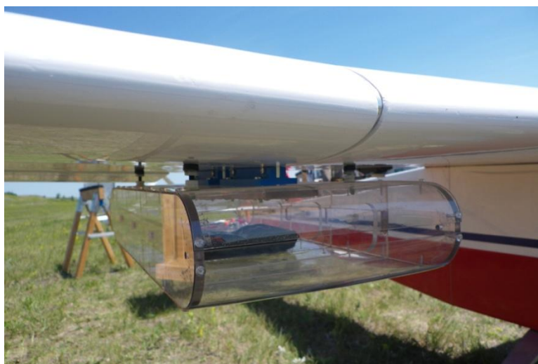
Figure 7. Wing pods installed in the Super Hauler.
