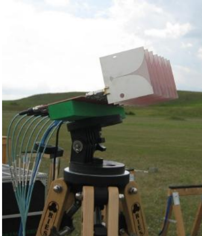
Figure 1: 5.8 GHz Phase Array Proof of Concept System
