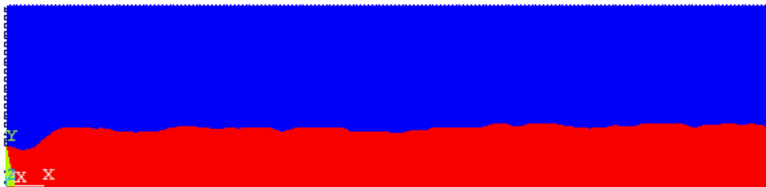
Figure 30: Valley of oscillation displacement amplitude at axisymmetric boundary location, Flotran volume fraction contour plot
