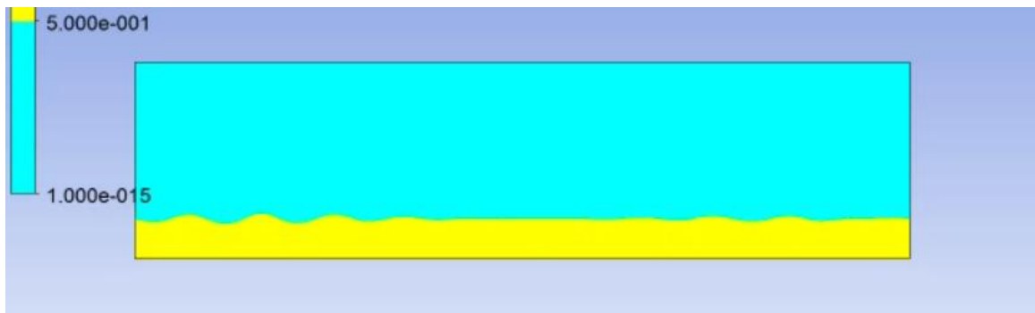
Figure 53: Standing waves beginning to form at boundaries and propagate across fluid body, CFX
