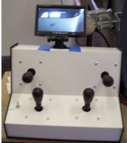
Figure 61: Control Box with Video Monitor on Top
