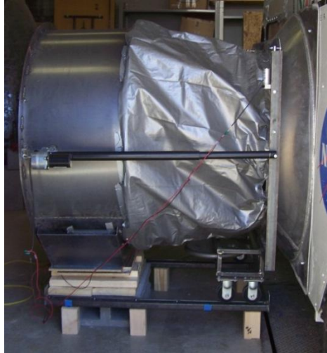
Figure 59: Tunnel with Mock-Up Bladder Docked with the PER
