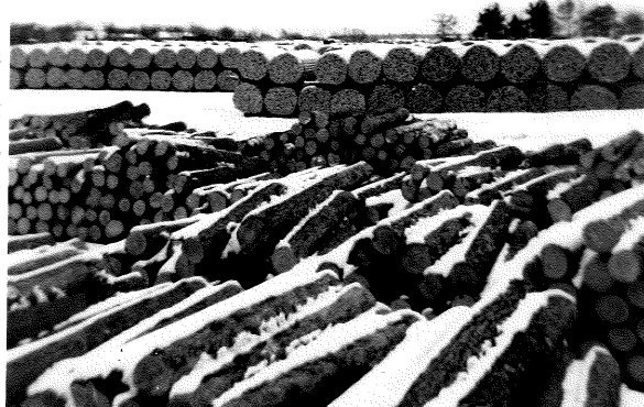
Figure 12. POST STOCKPILE. (Foreground--unpeeled posts ready for processing. Background--posts are peeled, ends finished, banded and ready for shipment. Wheeler Lumber and Bridge Supply, Cass Lake, Minnesota).
