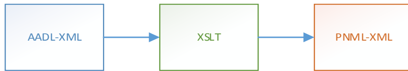
Figure 2. The conversion of AADL-XML to PNML via XSLT.
